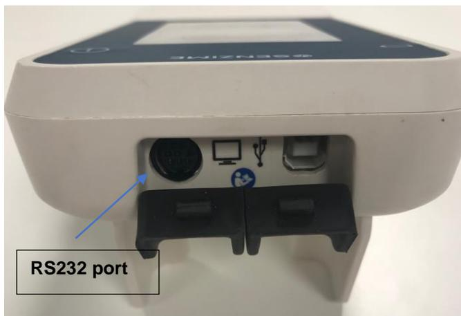
**Figure 3.** The RS232 port of TetraGraph Monitor allows external devices to be connected.
